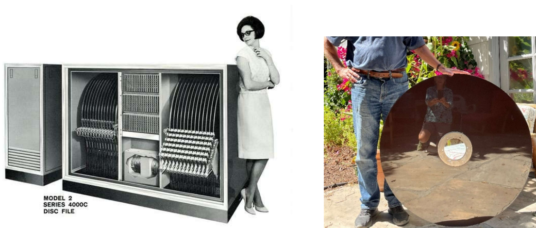
Left: The 205MB 39" Bryant Model 2. Right: A Bryant disk from my collection
