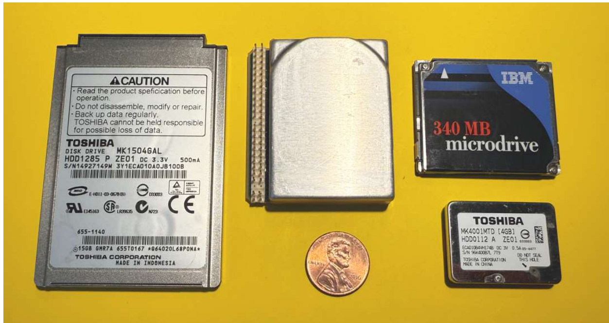
Small form factor HDDs from my collection (15GB Toshiba 1.8", 20MB HP 1.3", 340MB IBM 1.0", and 4GB Toshiba 0.85")
