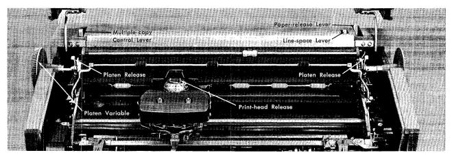
Figure 8. Impression and Form Controls
