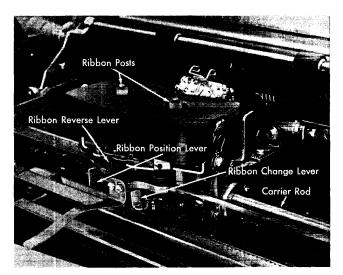
Figure 9. Console Printer Ribbon
