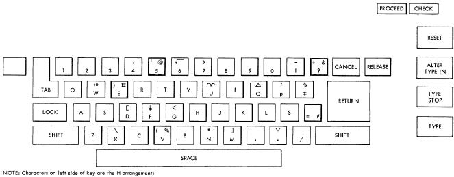
NOTE: Characters on left side of key are the H arrangement; characters on right side of key are the A arrangement.
