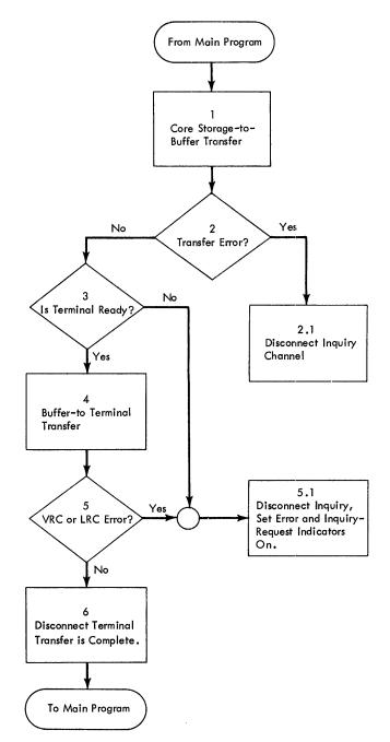
Figure 15. Programmed Write to a Terminal
