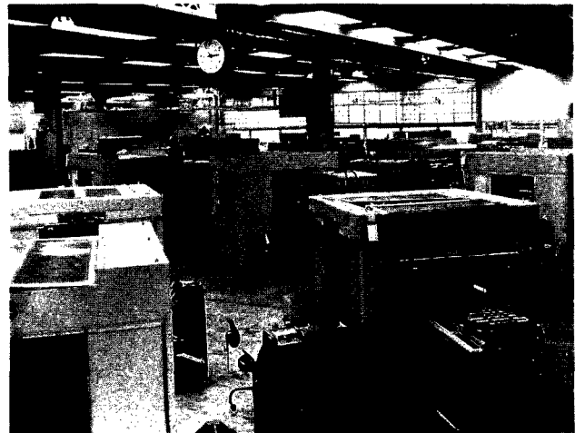
Fig. 5.—Gardner-Denver automatic wire wrap machines used to fabricate panels.
