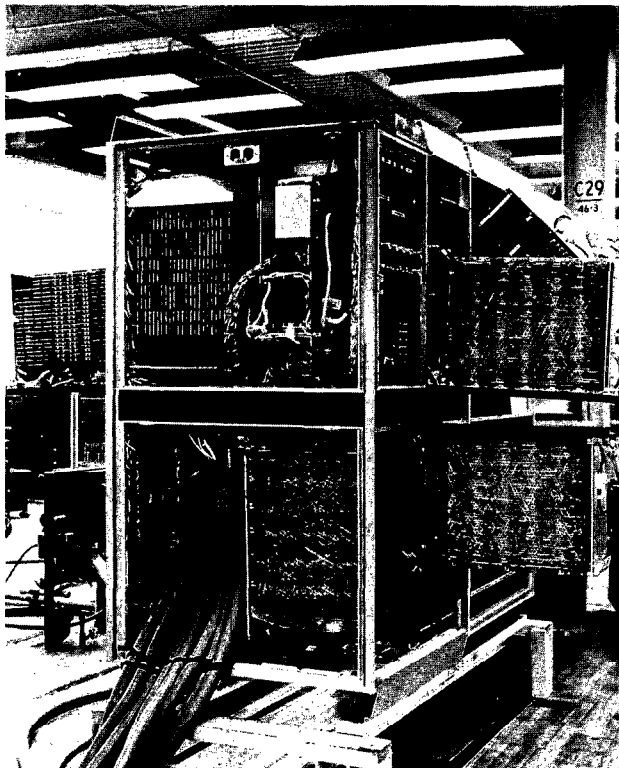
Fig. 4.—Wired panels in the IBM 1401 Data Processing System Central Processing Unit.
