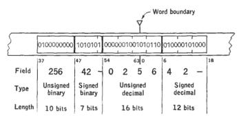
FIG. 4.2. Data units for fixed-point arithmetic.
