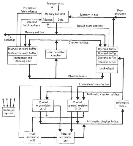
FIG. 14.4. Computer units and bus system.
