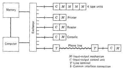
FIG. 12.3. Input-output connections to computer.
