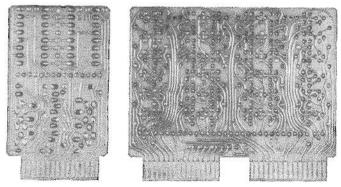
FIG. 14.20. Single and double circuit cards. Front and rear views.
