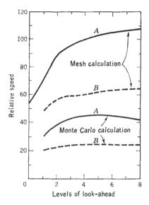
FIG. 15.1. Computer speed vs. number of levels of look-ahead. Four main memories, 2.0  $\mu$ sec; two fast memories, 0.6  $\mu$ sec; for two sets of arithmetic speeds:
