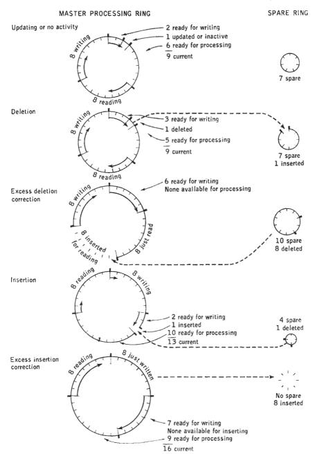
FIG. 11.10. Control-word diagram for file maintenance.
