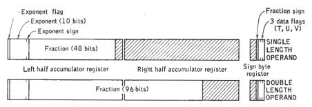
FIG. 8.4. FLP accumulator formats. Shaded areas are left undisturbed.
