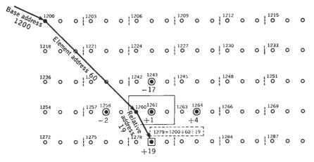
FIG. 11.1. Example of addressing of nearest neighbors in two-dimensional array. Example shows a  $6 \times 5$  array of three-valued elements, with relative addressing of the second value of one element and of its four nearest neighbors.
