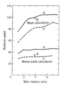
FIG. 15.2. Computer speed vs. number of main memory units. Four levels of look-ahead; arithmetic-unit time 0.64  $\mu$ sec; instruction-unit time 0.6  $\mu$ sec. A: instructions in separate 0.6- $\mu$ sec memory; B: instructions in separate 2.0- $\mu$ sec memory; C: instructions and data sharing same 2.0- $\mu$ sec memory.
