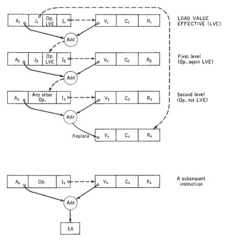
FIG. 11.8. Indirect addressing and indirect indexing. If  $A_4 = 0$ ; indirect addressing. If  $A_4 \neq 0$ ; indirect indexing. LOAD VALUE EFFECTIVE can be repeated automatically any number of times; two levels of indirect addressing are shown; last level is one where operation code encountered is something other than LVE.
