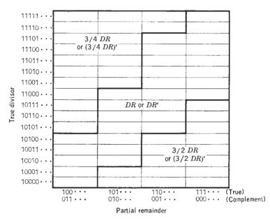
FIG. 14.11. Table for selecting divisor multiple. Select complement-divisor multiple if partial remainder is true. Select true-divisor multiple if partial remainder is a complement.
