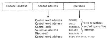
FIG. 12.1. Principal parts of input-output instructions.
