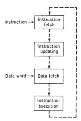
FIG. 14.2. Sequential operation.
