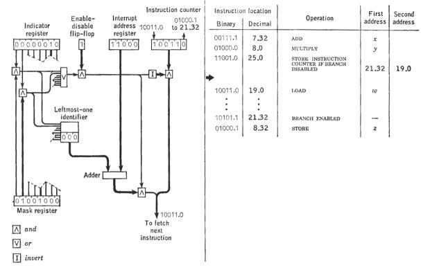
FIG. 10.4. Program-interrupt example. Interrupt subroutine with further interrupts inhibited.
