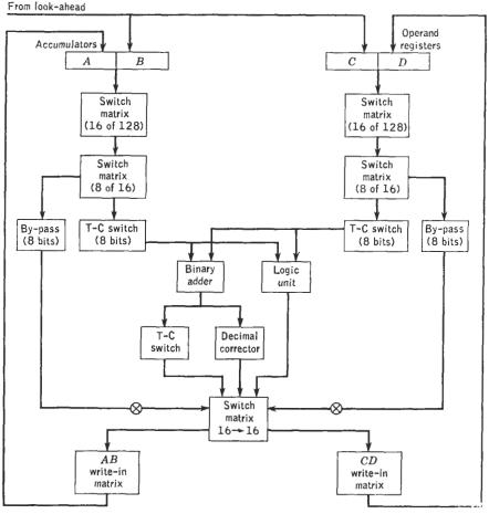
FIG. 14.6. Serial arithmetic unit. T-C: true-complement.
