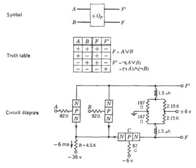
FIG. 14.17. Current-switching circuit, NPN.
