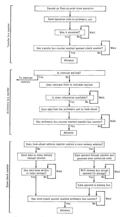
FIG. 15.10. Transfer-bus, arithmetic-bus, and store-check counter advance sequences for floating-point store-type operations.
