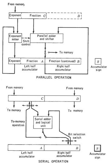
FIG. 3.2. Simplified register structure of arithmetic unit.
