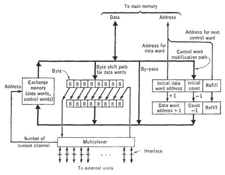
FIG. 16.1. Data-flow paths of exchange.
