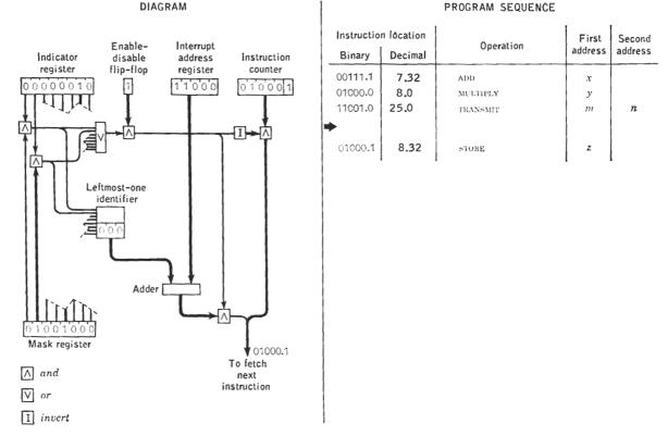
FIG. 10.3. Program-interrupt example. One-instruction fix-up.
