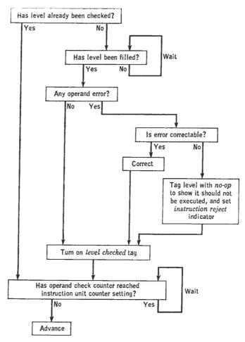
FIG. 15.8. Operand-check counter advance sequence.
