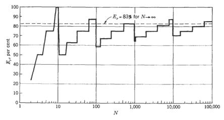
FIG. 5.2. Relative efficiency of decimal and binary number systems.  $E_r = b_2/b_{10}$ , where  $b_2$  ( $b_{10}$ ) is the least number of bits in the binary (decimal) representation of N.
