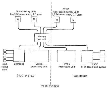
FIG. 17.1. Nonarithmetical extension of the 7030.
