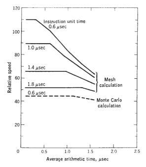
FIG. 15.3. Computer speed vs. arithmetic times for various instruction-unit times. Four levels of look-ahead; four units of 2.0-µsec memory; two units of 0.6-µsec memory.
