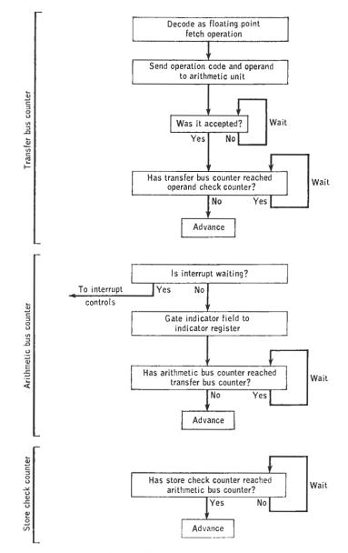
FIG. 15.9. Transfer-bus, arithmetic-bus, and store-check counter advance sequences for floating-point fetch-type operations.
