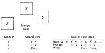
FIG. 11.9. Read-process-write chain.
