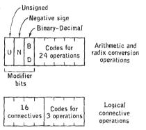
FIG. 7.2. Details of VFL operation codes.
