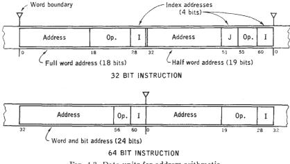
FIG. 4.3. Data units for address arithmetic.
