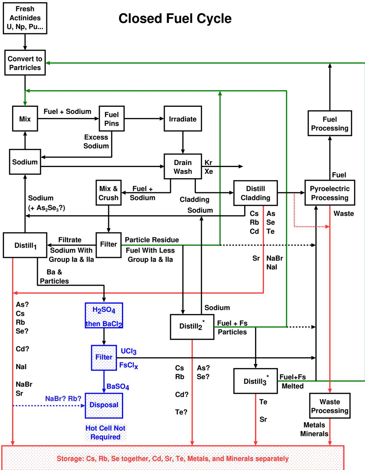
Figure 3: Closed Fuel Cycle
